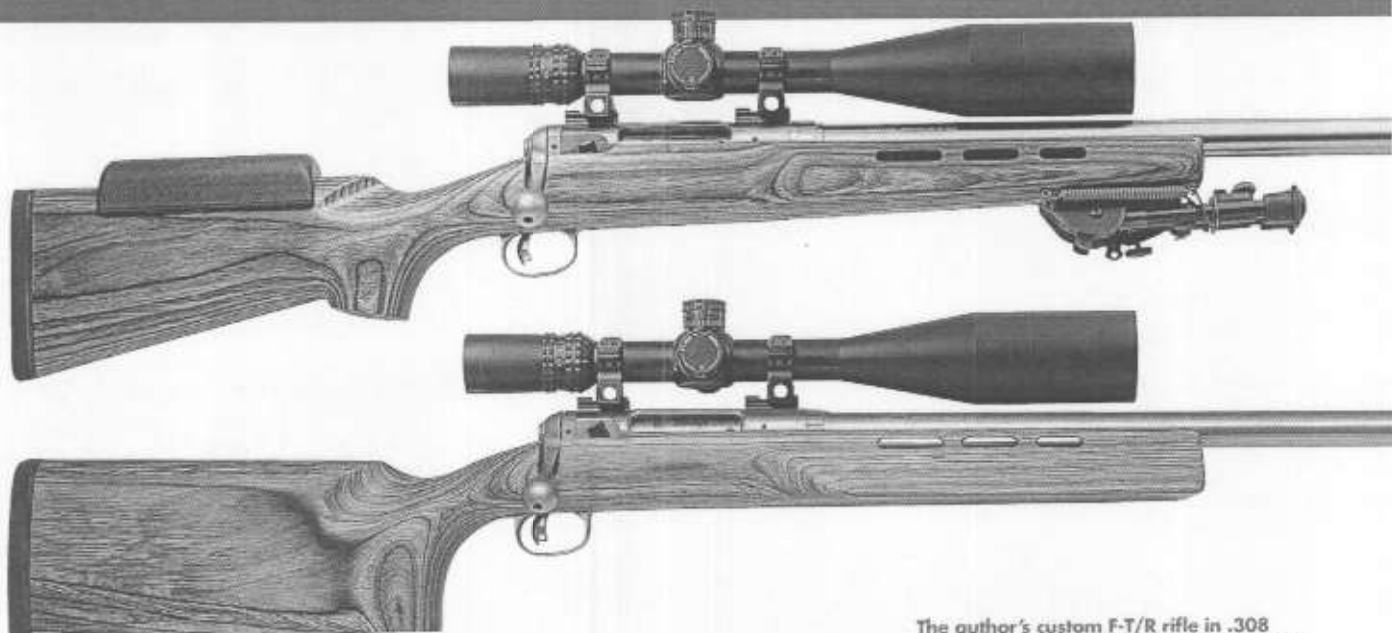
The author's custom F-T/R rifle in .308 Win. features a single-shot Lawton action, 30-inch barrel, McRees Precision aluminum stock, Harris bipod, Red-Tac rear bag and Nightforce NXS 5.5-22X56 scope.
